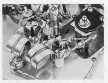
Figure 2. View of the harmonic generator incorporating the circuits of Figure 1.
